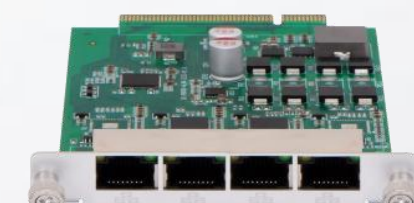
Four Gigabit Ethernet port
